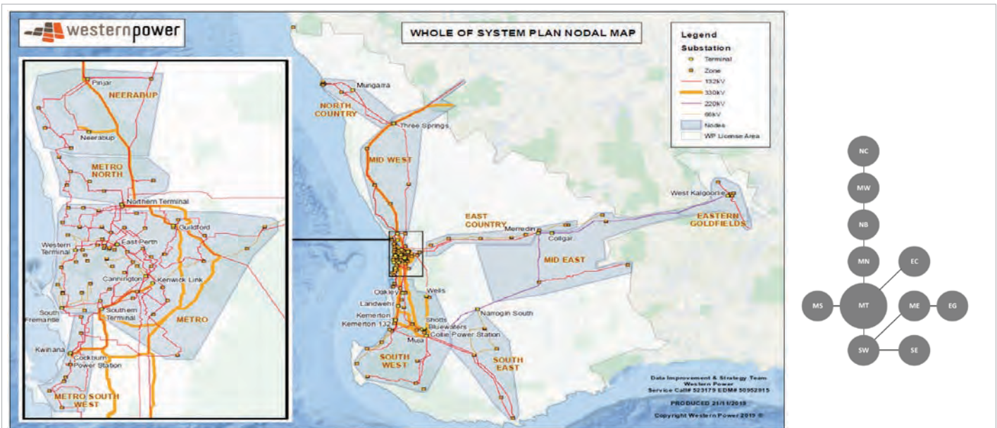
Figure 3.3 Map & schematic diagram of nodes being modelled in the Whole of System Plan. Images courtesy of Energy Policy WA. The maps on left indicate the HVAC lines divided into areas called nodes. On right is a schematic diagram of how these nodes are interconnected.
