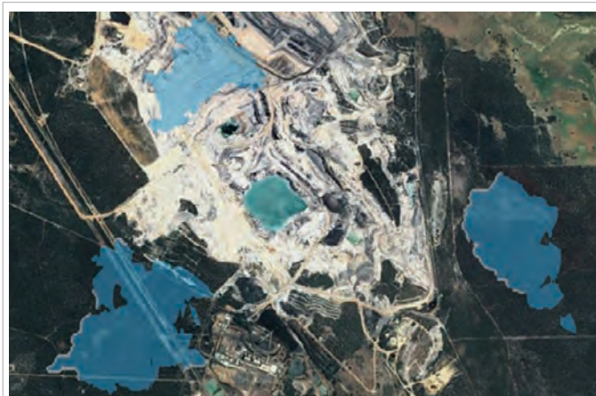
Figure E.2 Conceptual Pumped Hydro installations in repurposed Collie coal mine indicating three potential upper pond locations and a lower pond in the central of the image. Image provided by Professor Andrew Blakers for this report (A. Blakers, 2020).
